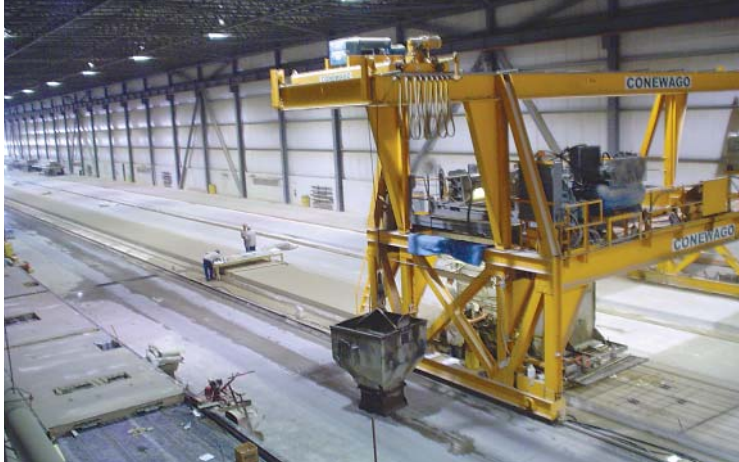
100,000 sq. ft. Conewago precast production facility features Spancrete® hollow-core plank and wall panel extrusion system and full PCS Computer Control System from ACS. Fill time for one 800-foot casting bed has been cut by nearly 50% thanks to improved control.
