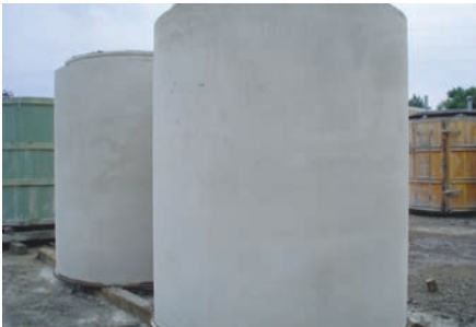
Proof on site – Virtually overnight, the PCS control system eliminated "bughole" cosmetic defects from pipe and other products through improved component proportioning accuracy and batching consistency. Customers noticed the improvement immediately.
