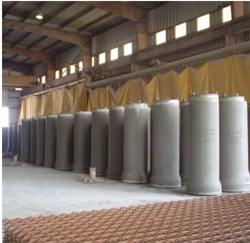
Newly produced concrete pipe cures indoors at Hanson's La Feria, Texas, plant. The entire plant is run by a single PCS Control System from ACS, providing advanced automation, complete documentation, and point-and-click control.
